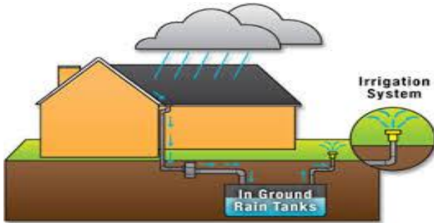
Image 6.14. Shows harvesting rain water to reduce surface runoff. Source: Field survey, (2025)
