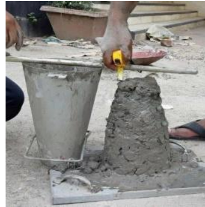
Figure 4. Slump test
