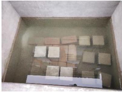
Figure 6. Curing into Salt Water
