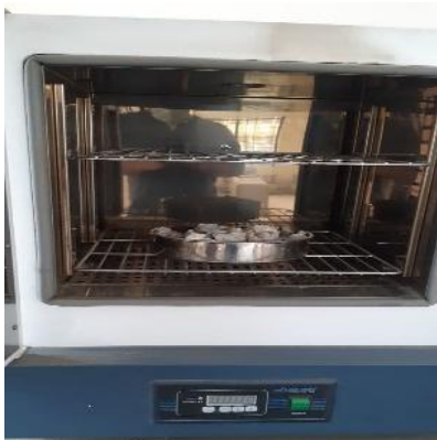
Figure 2. Absorption Capacity Test
