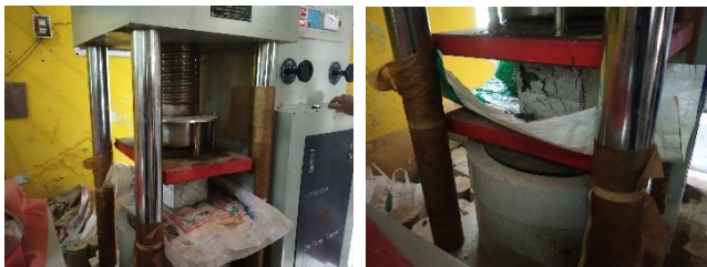
Figure 8. Compressive Strength Testing
