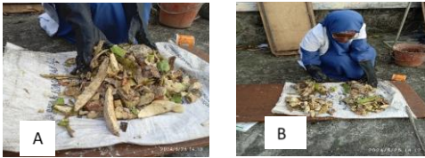
Figure 4. Cone shaping (A) and quatting (B) of waste
