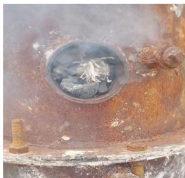
Figure 5. Ignition of the gasifier
