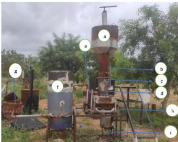
a: power area; b: pyrolysis area; c: combustion area; d: reduction area; e: cyclone area; f: heat exchanger; g: glow; h: ashtray; i: crank
