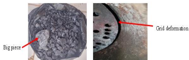
Figure 11. Charcoal residues and ash disposal grate
