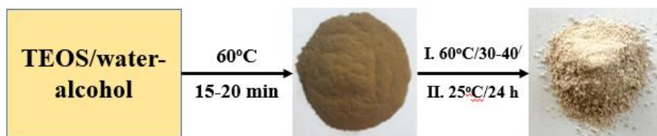
Figure 1. Scheme for Obtaining a Silica-Bentonite Composite
