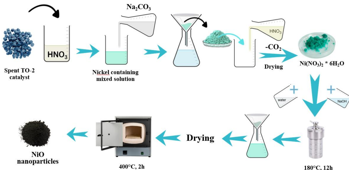
Figure 1. Scheme for obtaining nanodispersed NiO based on spent catalyst TO-2
