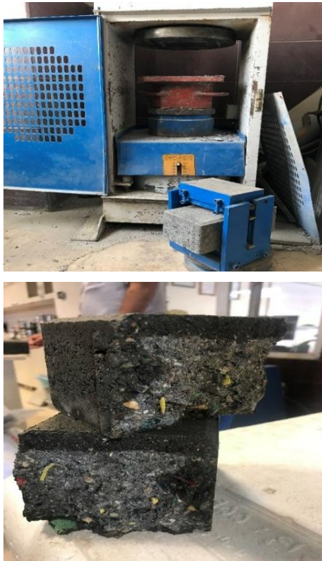
Figure 6. Tensile strength test machine and Brazilian enclosure and flooring sample after performing tensile strength test
