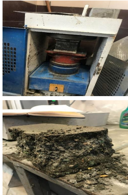
Figure 4. Sample after compressive strength test
