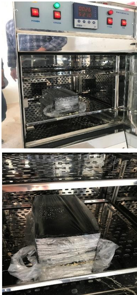
Figure 16. Melting and ice test of concrete floor containing VP particles
