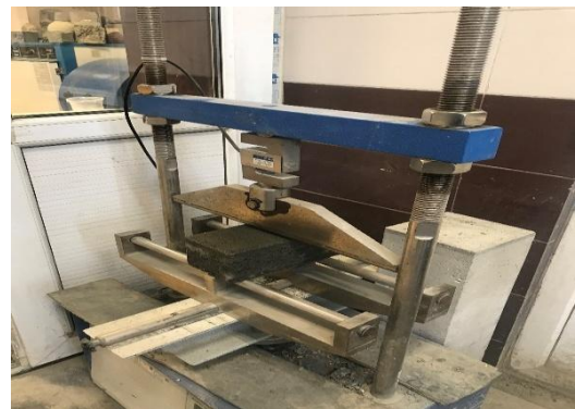
Figure 8. Flooring under flexural strength test
