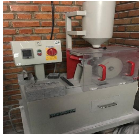
Figure 12. Wide wheel abrasion tester with sample
