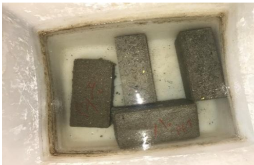
Figure 14. Test to determine the water absorption of the entire concrete floor containing VP particles
