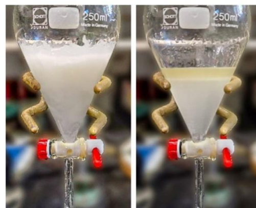
Figure 4. Phase separation of soybean oil-based biodiesel from 10% NaCl solution. The parts on the left and right are for untreated, and pre-treated soybean oil, respectively
