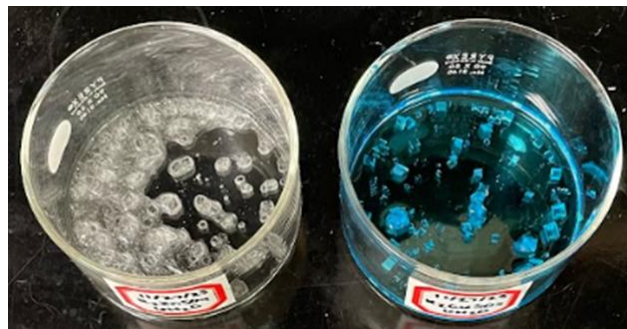
Figure 5. Crystals of two potassium double salts two days after synthesis. For each salt, a thin aqueous layer of solution remains. The colorless zinc salt and blue copper salt are shown from left to right
