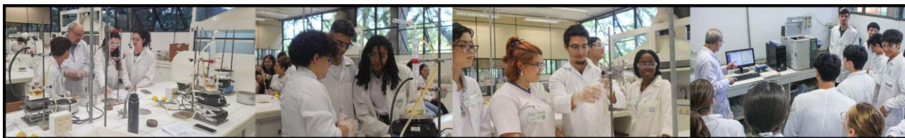
Figure 4. The students and the staff working. The parts from left to right show: determination of the AV of the WCO by acid-base titration; assembling glassware for the experiment; volumetric measurement of ethanol, and demonstration of gas chromatographic analysis
