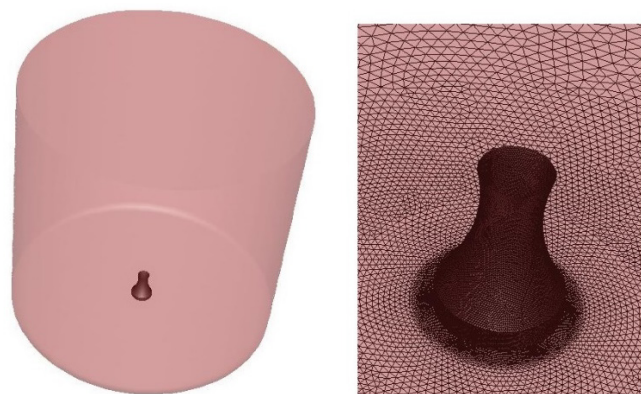
Figure 1. Geometry of studied dry cooling tower and simulation domain
