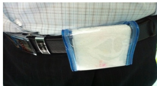
Figure 3. Sensor module is installed with the belt at the body waist
