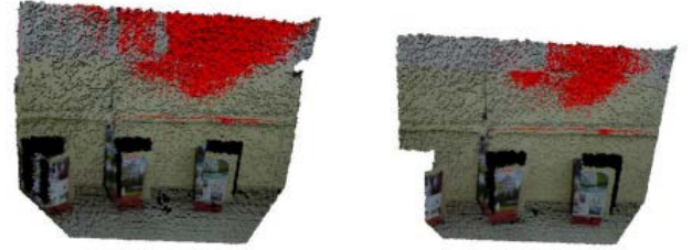
Figure 9. 3D cloud images combined by RGB and depth images of the room space
