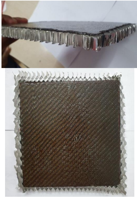
Figure 4. Prepared sandwich panel
