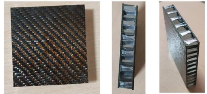
Figure 9. Edgewise compression test samples
