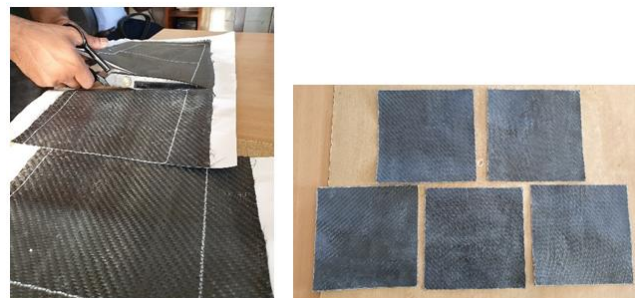
Figure 2. Cut bi-directional 2x2 carbon twill with dimensions 165\text{mm} \times 165\text{mm}
