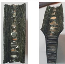
Sample 3 (End failure)
