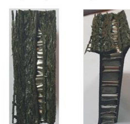
Sample 4 (End failure)
