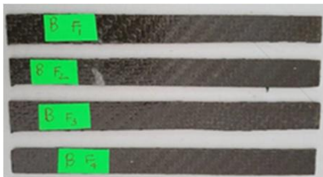
Figure 13. Cut CFRP samples for UL94 fire retardant test
