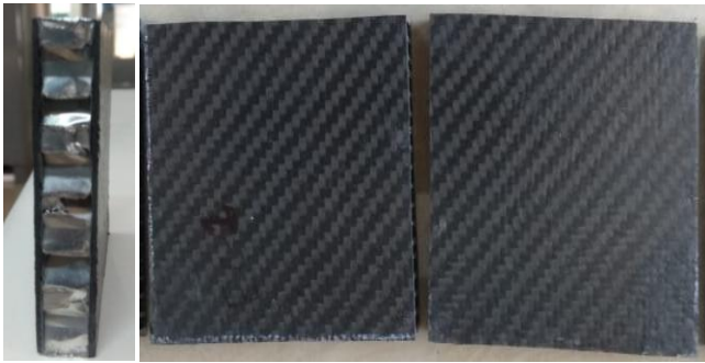
Figure 11. Flatwise compression test samples
