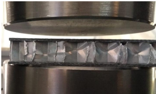
Figure 12. Flatwise compression test ready for testing
