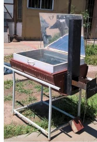
**Figure 7.** View of the oven with the open brazier ready to place the embers
