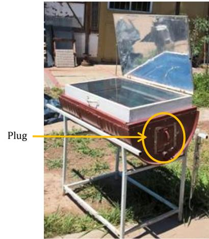
Figure 8. Oven with the “plug” utilized when operates only with solar energy (on clear days)
