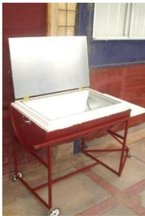
Figure 1. Drum solar oven with mobile stand
