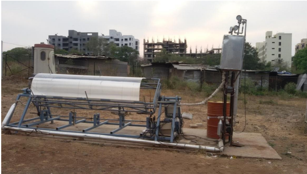
Figure (1b). Photograph of Fresnel lens solar concentrating system
