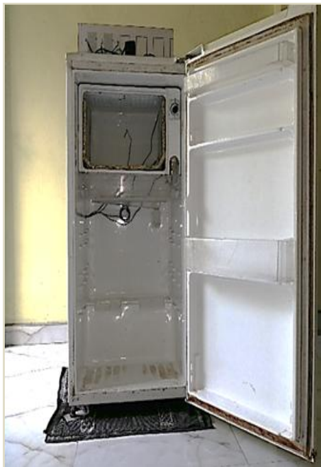
Figure 1(a). Refrigerator showing PCM installation
