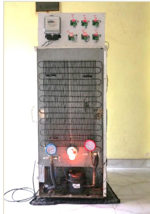
Figure 1(b). Back of Refrigerator showing instrumentation
