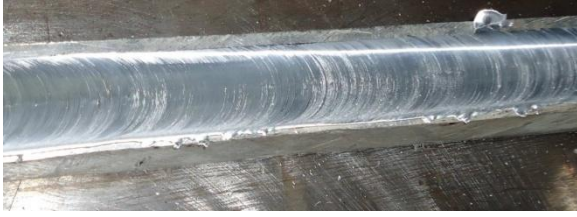
Figure 3. Picture of as-processed plate with one pass at 500 rpm, 20 mm/min
