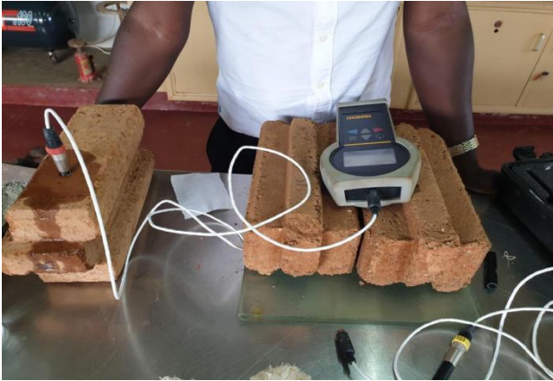
Figure 4. Measurement of thermal properties
