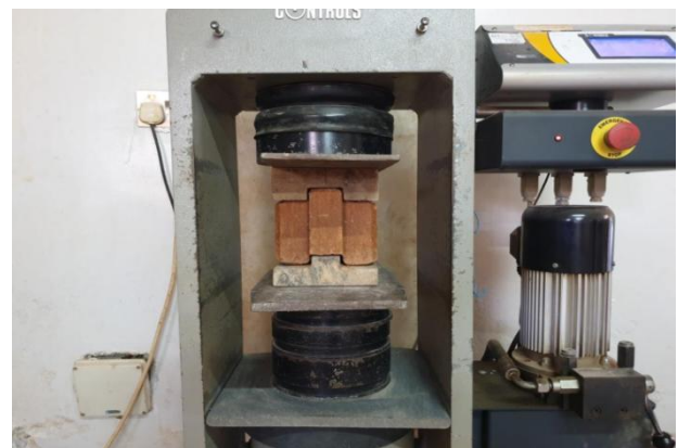
Figure 3. Compressive strength test setup
