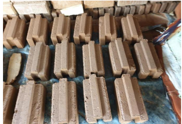
Figure 2. Air curing of Interlocking stabilised soil block samples
