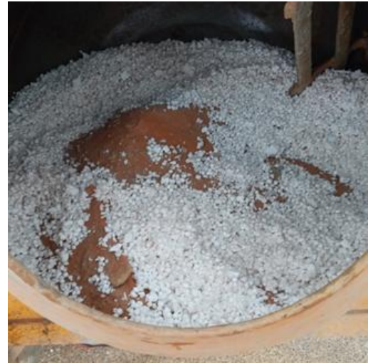
Figure 2. Processed expanded polystyrene waste being mixed with soil
