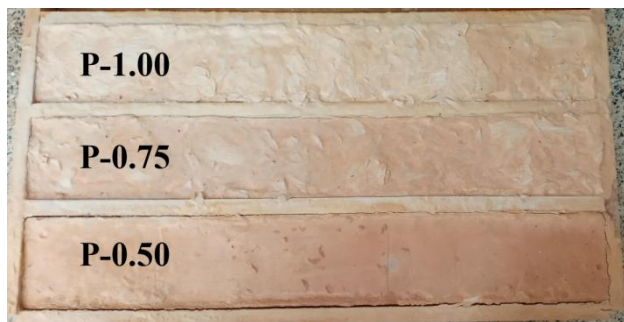
Figure 13. Shrinkage test: soil-cement with polyethylene fibers
