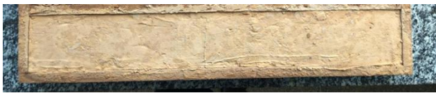
Figure 16. Shrinkage test: soil-cement with EPS + polyethylene fibers
