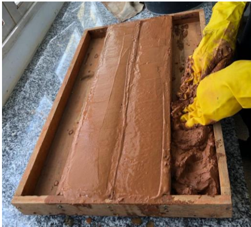
Figure 5. Accommodation of mixtures in the shrinkage test box
