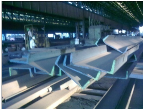
Figure 1. ISMB 250 Channels of IS 2062 E410 grade B steel at Heavy Structural Mill, ISP
