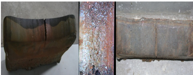
Figure 3. Typical cracks observed on the rolled blooms
