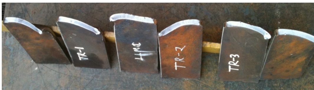
Figure 3. Fractured surfaces of DWTT tested specimens
