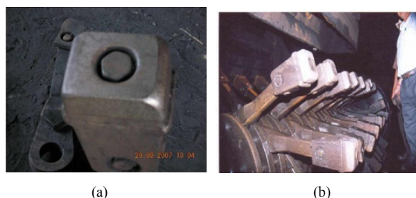
Figure 10. New Hammers after use of 2000 hrs (a)- Close up view, (b)- Assembled in mill
