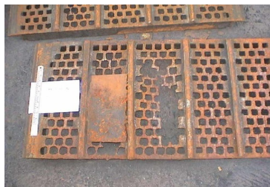
Figure 11. Screen made from 4 mm thick carbide deposited layer
