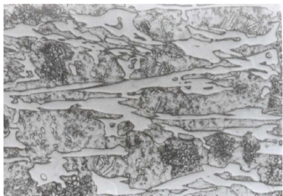
Figure 7b. Microphotograph of new Hammer material-1000X
