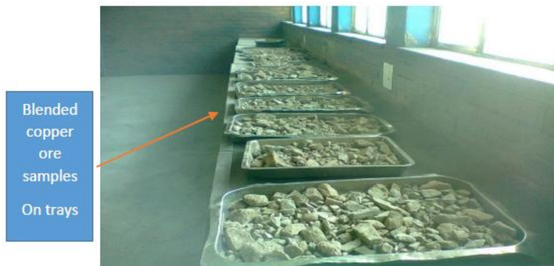
Figure 3. Samples being cooled after drying below 100°C
