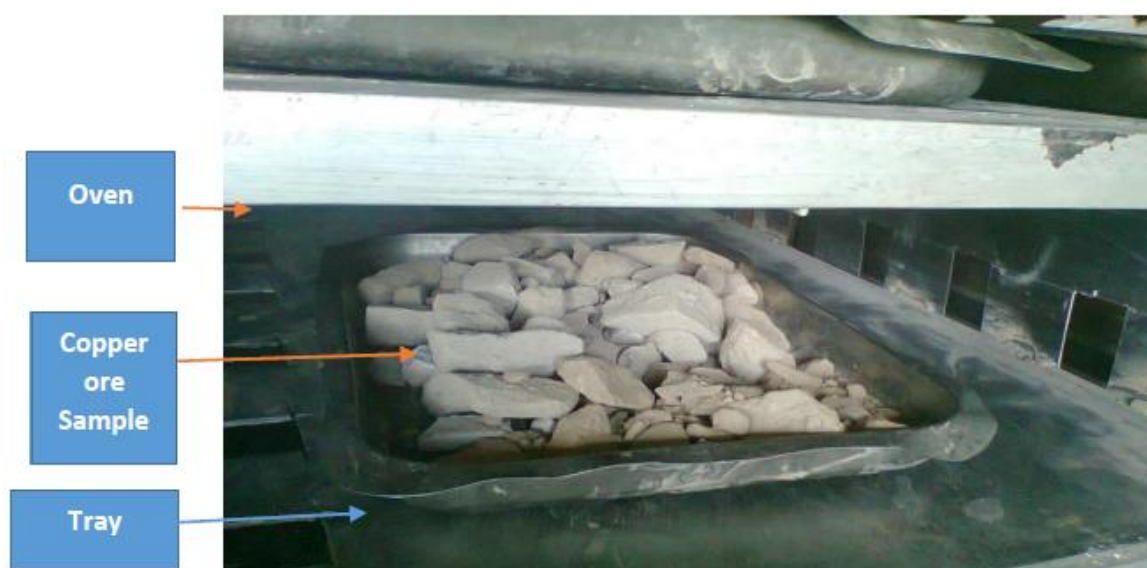
Figure 2. Drying of the samples in the oven below 100°C (Done below 100°C to avoid oxidation of the ore samples)
