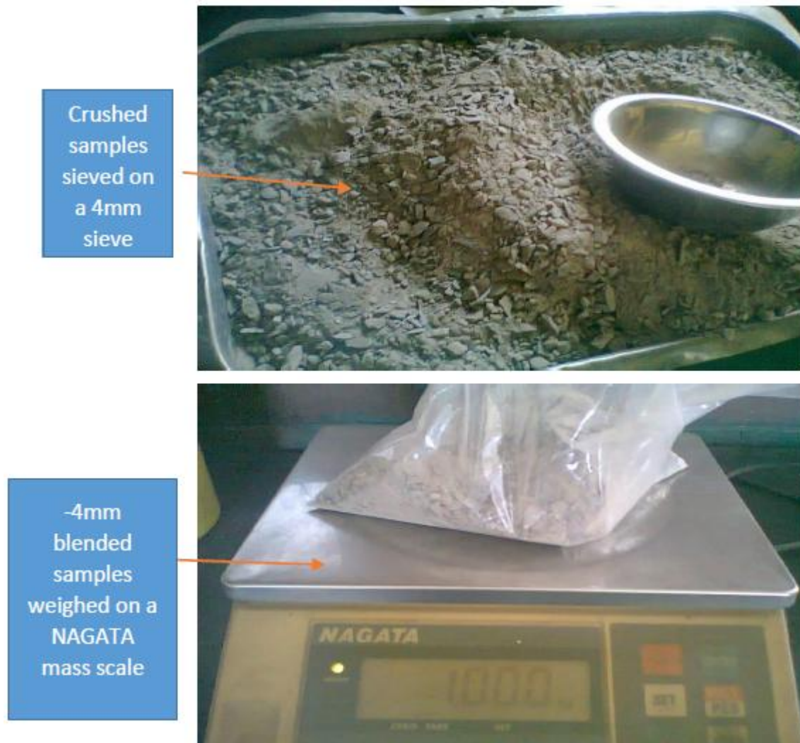
Figure 4. -4mm sieved sample ores crushed and weighed (1000g)
