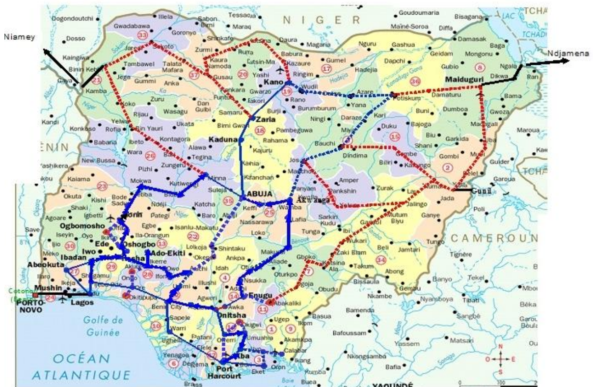
Figure 4. Glo fiber optic backbone networks [6]
