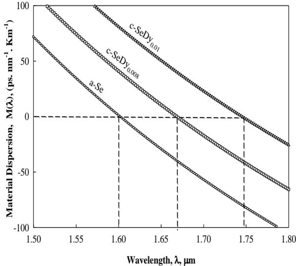
**Figure 8.** Variation of the material dispersion versus wavelength for the studied films
