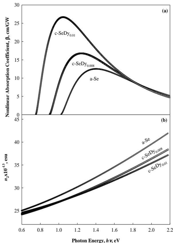
**Figure 9.** Dependence of nonlinear absorption coefficient,  $\beta$  (a) and second order refractive index,  $n_2$  (b) on the incident photon energy,  $h\nu$  for the studied films
