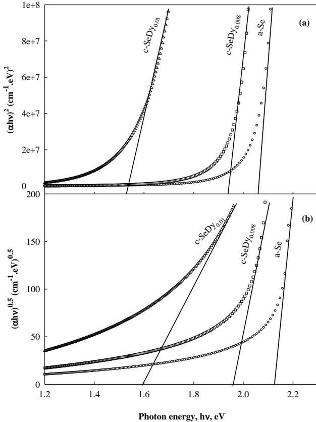
**Figure 5.** Tauc's plots for determining the optical energy gap of direct (a) and indirect (b) transitions for films investigated
