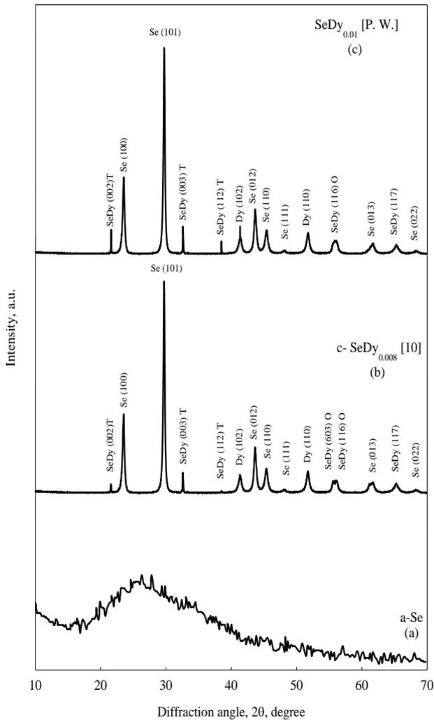
**Figure 1.** XRD pattern for a-Se (a), c-SeDy<sub>0.008</sub> [10] (b) and the present work [P. W.] of SeDy<sub>0.01</sub> (c) thin films. It should be noted that the diffraction pattern of c-SeDy<sub>0.008</sub> [10] is added to the figure for the sake of comparison
