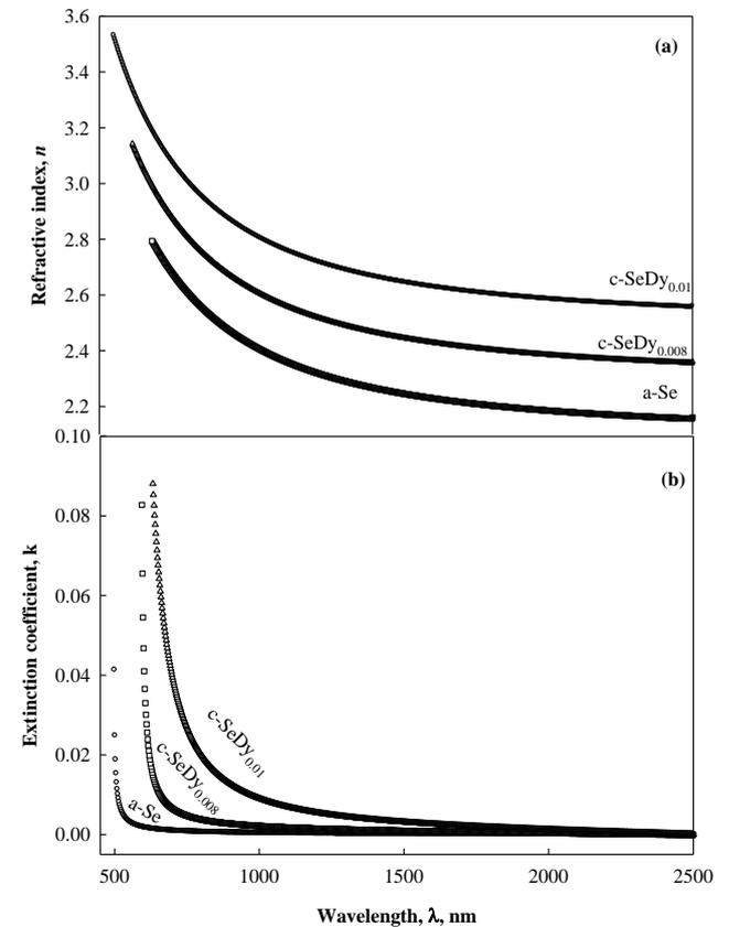
**Figure 2.** Variation of refractive index ( $n$ ) (a) and extinction coefficient ( $k$ ) (b) with wavelength ( $\lambda$ ) for the studied a-Se, c-SeDy<sub>0.008</sub> and c-SeDy<sub>0.01</sub> thin films
