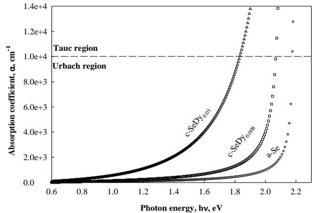
**Figure 4.** The calculated absorption coefficient ( $\alpha$ ) as function of photon energy ( $h\nu$ ) for the studied films. The dashed horizontal line differentiates between the Tauc and Urbach regions
