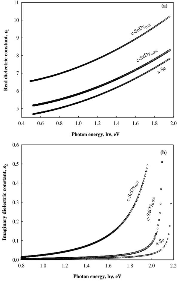
**Figure 6.** Real (a) and imaginary (b) parts of the dielectric constant versus photon energy for the films investigated
