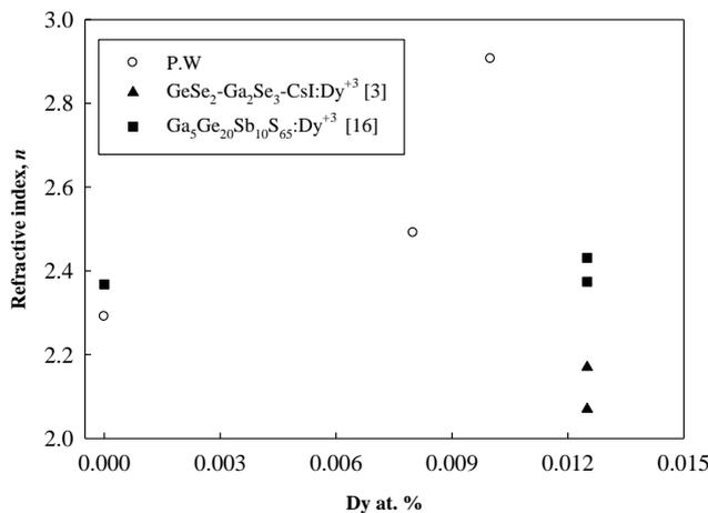
**Figure 3.** Variation of refractive index as a function of the doped Dy rare earth ions in at. % for the present work [P. W.] with those published in the literature such as  $\text{GeSe}_2\text{-Ga}_2\text{Se}_3\text{-CsI}:\text{Dy}^{+3}$  [3] and  $\text{Ga}_3\text{Ge}_{20}\text{Sb}_{10}\text{S}_{65}$  [16]
