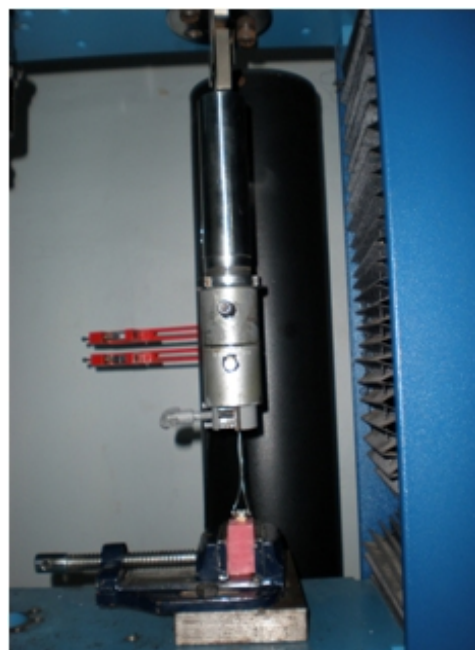
Figure 1. Universal testing machine experiment setup
