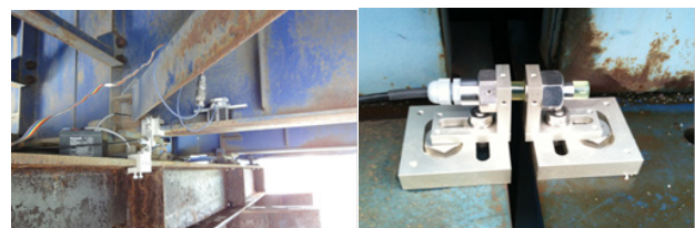
(h) Sensor measurement method for temporary bridge
