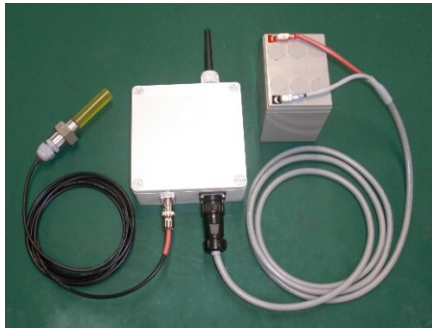
Figure 7. Piezoelectric vibration sensor for structural health monitoring system
