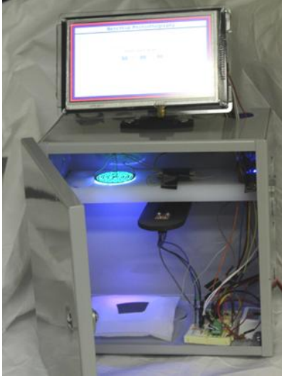
Figure 1. The benchtop photolithography tool
