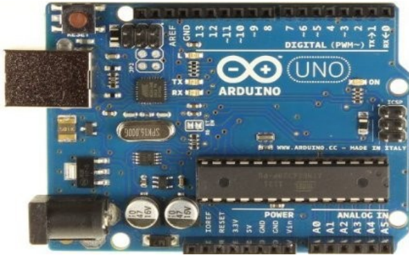
Figure 4. Arduino Board with In circuit serial programming (ICSP)
