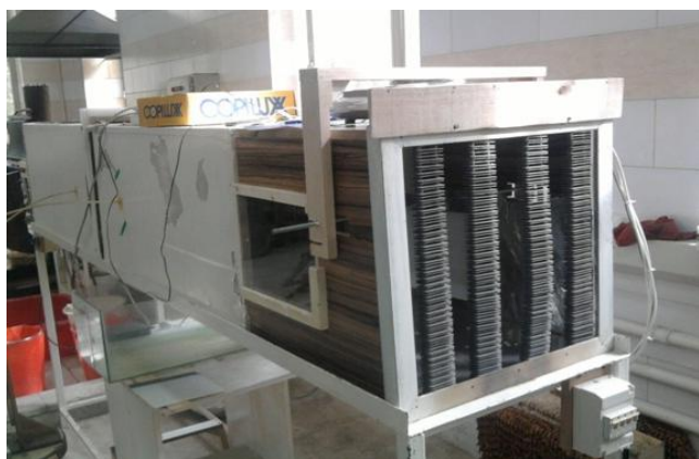
Figure 2. Wind tunnel used for tests
