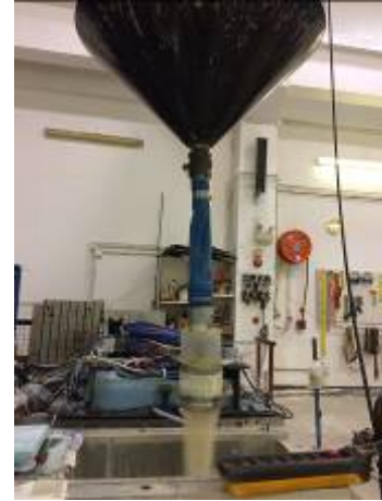
Figure 2. Sand layer pouring [25]
