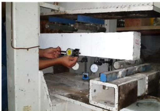
b. Flexure strength for beam samples
