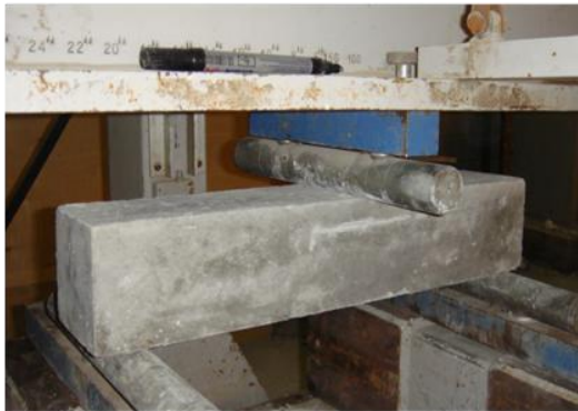
a. Flexure strength testing for prisms.
