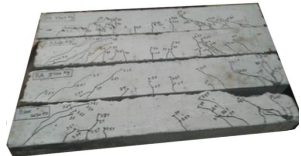
Figure 35. Crack patterns for self-curing beams cast using chloride attack after 28 days
