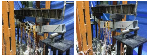
Figure 9. Testing the strength of Aluminum joints in different orientations under bending loading
