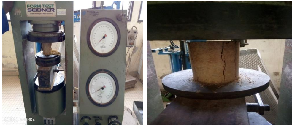
Figure 10. Compression test apparatus
