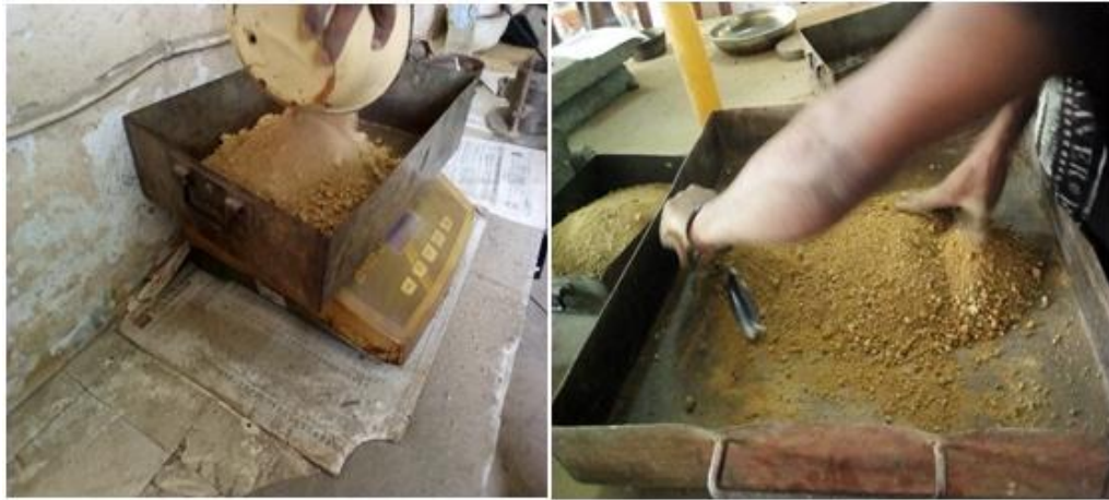
Figure 7. Weighing and mixing the soil
