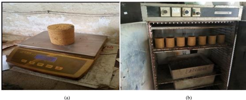
Figure 9. Weighing of the test piece (a). Test pieces produced and put to drying (b)
