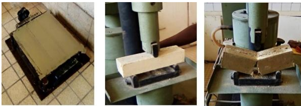
Figure 11. Bending test device
