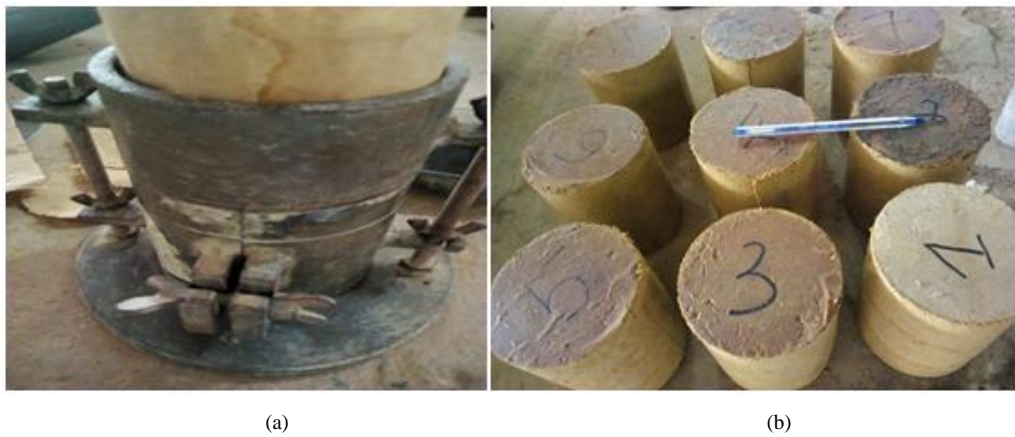
Figure 8. Preparations of test pieces (a). Test pieces produced and put to drying (b)
