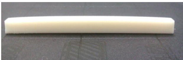
Figure 3. Warping of 3D printed part due to stress build-up
