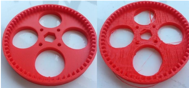
Figure 9. Parts A & B from left (part A) to right (part B) exhibiting variations in surface quality
