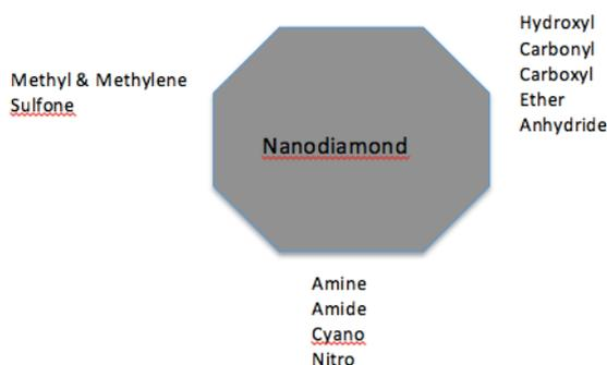
**Figure 4.** Common functional groups on the nanodiamond surface [56]
