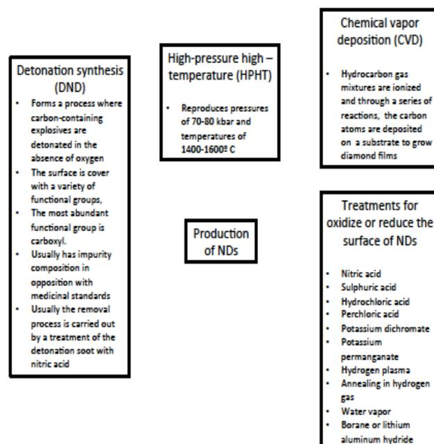
Figure 3. Production methods of nanodiamonds
