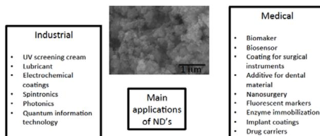
Figure 2. Main applications of NDs and SEM micrograph of commercial nanodiamonds purchased to Sigma-Aldrich
