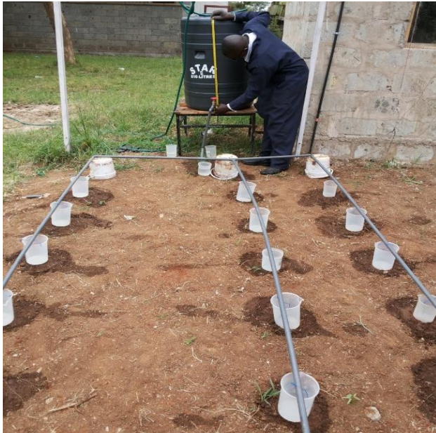
Figure 2. Layout of the system for discharge collection
