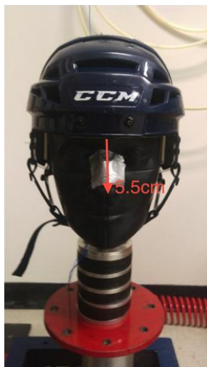
Figure 2. NOCSAE headform with properly fitted helmet. A distance of 5.5cm is measured between the brim of the helmet and the tip of the nose
