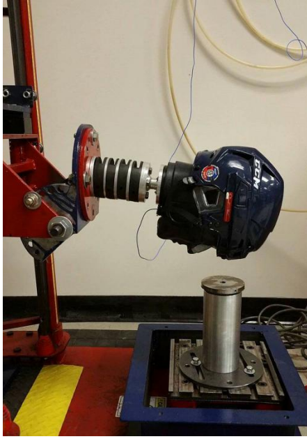
Figure 4. Drop system and impact anvil
