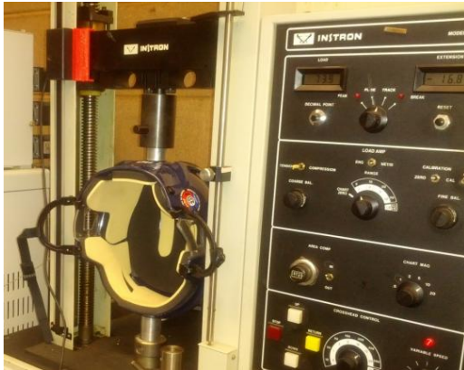
Figure 5. Instron 1000- test equipment for mechanical properties of materials
