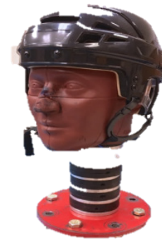
Figure 3. NOCSAE headform fitted with hockey helmet and mounted on mechanical neckform
